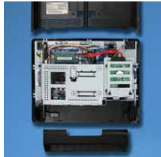
Tool-Free Access to RAM Optimizes Serviceability
